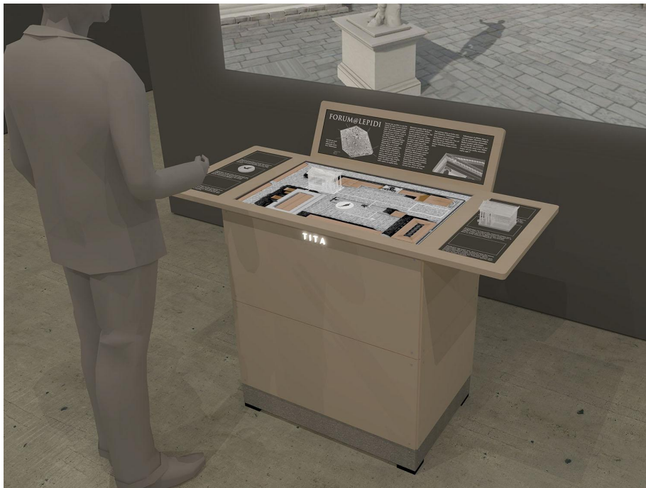
Fig. 2. Tangible/multi-touch interaction surface, tangible trays and illuminated signage.
